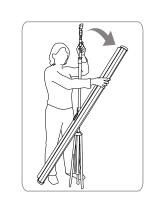
Lift the screen using the ring and place onto the top hook.
