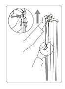
Raise the top hook using the coloured button to release the top locating pin.
