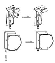
Ensure the wall bracket is secured to the casing of the screen before hanging.
