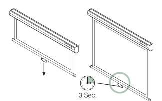
Retract the screen by pulling down the handle and then let go of it. The screen will retract at a controlled speed.
