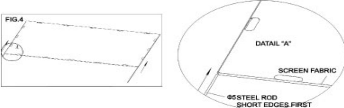
5. Put the prepared screen fabric to the frame. Use the spring hook to fix them. Short edges first. Check and adjust to ensure flatness.
