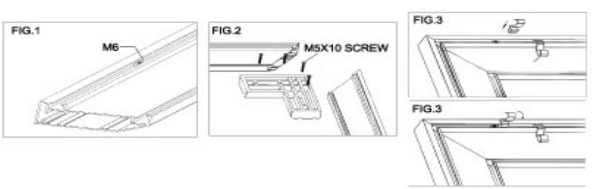
3. Insert the spring hooks into the frame slot, and turn 90°.fig.3
