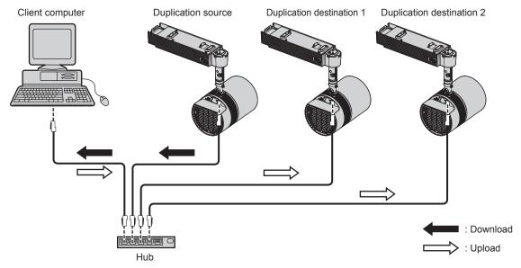
(Example) Illustration of connecting via wired LAN
