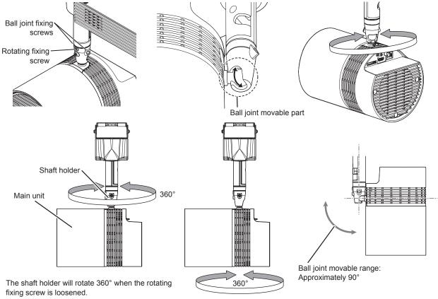
Move the ball joint movable part to the direction to tilt the main unit.
