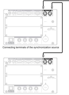
Connecting terminals of the synchronization target
