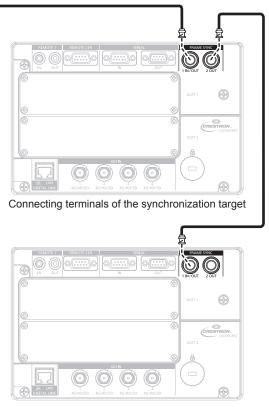
Connecting terminals of the synchronization target
