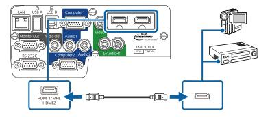
If you have problems hearing audio through the HDMI connection, connect one end of a commercially available 3.5 mm stereo mini-jack audio cable to the projector's Audio port and the other end to your computer's audio out port. Select the input port you connected to from the HDMI1 Audio Output or HDMI2 Audio Output setting in the projector's Extended menu.
