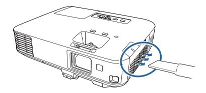
You can remove the air filter so that you can clean both sides. Do not rinse the air filter in water, or use any detergent or solvent to clean it.
