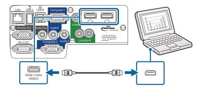
If you have problems hearing audio through the HDMI connection, connect one end of a commercially available 3.5 mm stereo mini-jack audio cable to the projector's Audio port and the other end to your computer's audio out port. Select the input port you connected to from the HDMI1 Audio Output or HDMI2 Audio Output setting in the projector's Extended menu.
