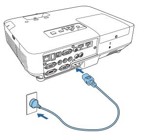
The projector's power light turns blue. This indicates that the projector is receiving power, but is not yet turned on (it is in standby mode).
