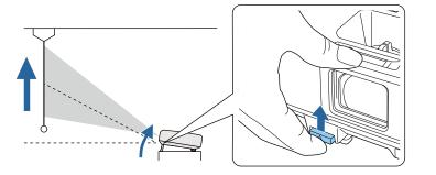
The foot extends from the projector. You can adjust the position up to 14 degrees.
