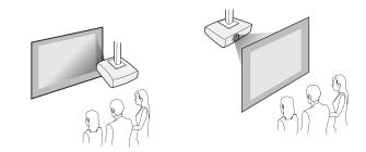
When projecting from the ceiling or from the rear, make sure you select the correct **Projection** option in the projector's **Extended** menu.
